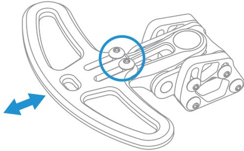
Reach can be adjusted by slightly loosening the two screws highlighted as the right picture and the two on the opposite side of the shifter as pointed by the small arrows, then rotating the lever body upwards/downwards. You may need to apply a bit of force.
